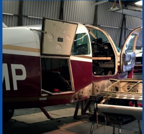
Repairing the walkway & riveting.
